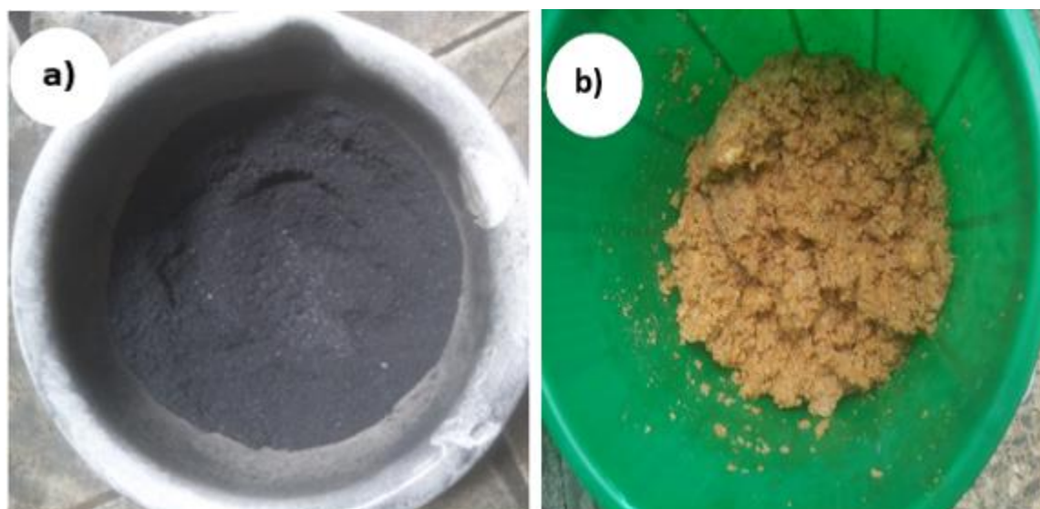
Figure 8. a) was the crushed Biochar while, b) was crushed food waste before being liquidized
