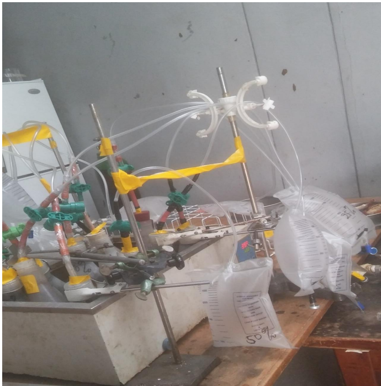
Figure 9. Set-up of lab experiment for biogas production through Anaerobic digestion
