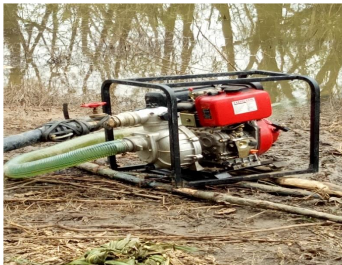
Figure 3. 6 Diesel water pumping system at Gashora site
