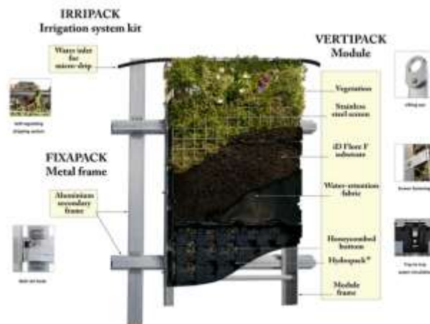
Figure 13 :Details of vegetal wall
