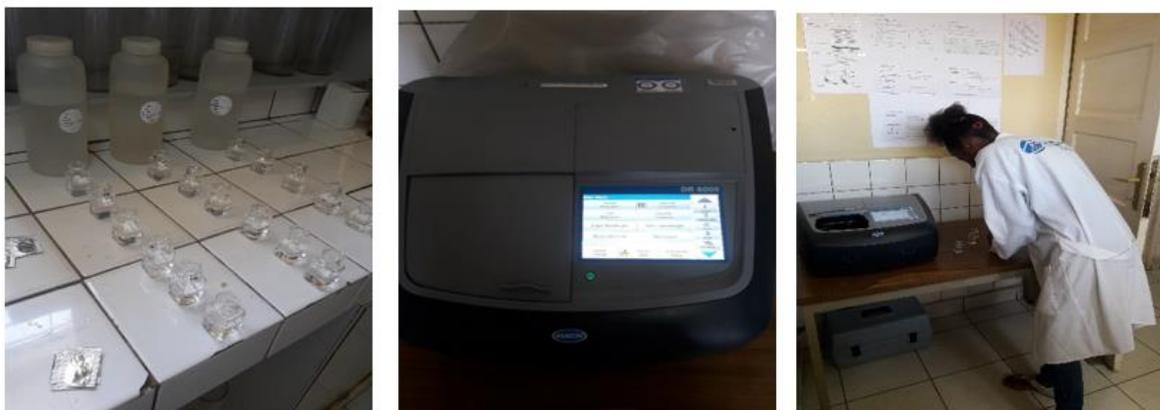
**Figure 3.2. Sample Cells and Spectrophotometer Machine**
