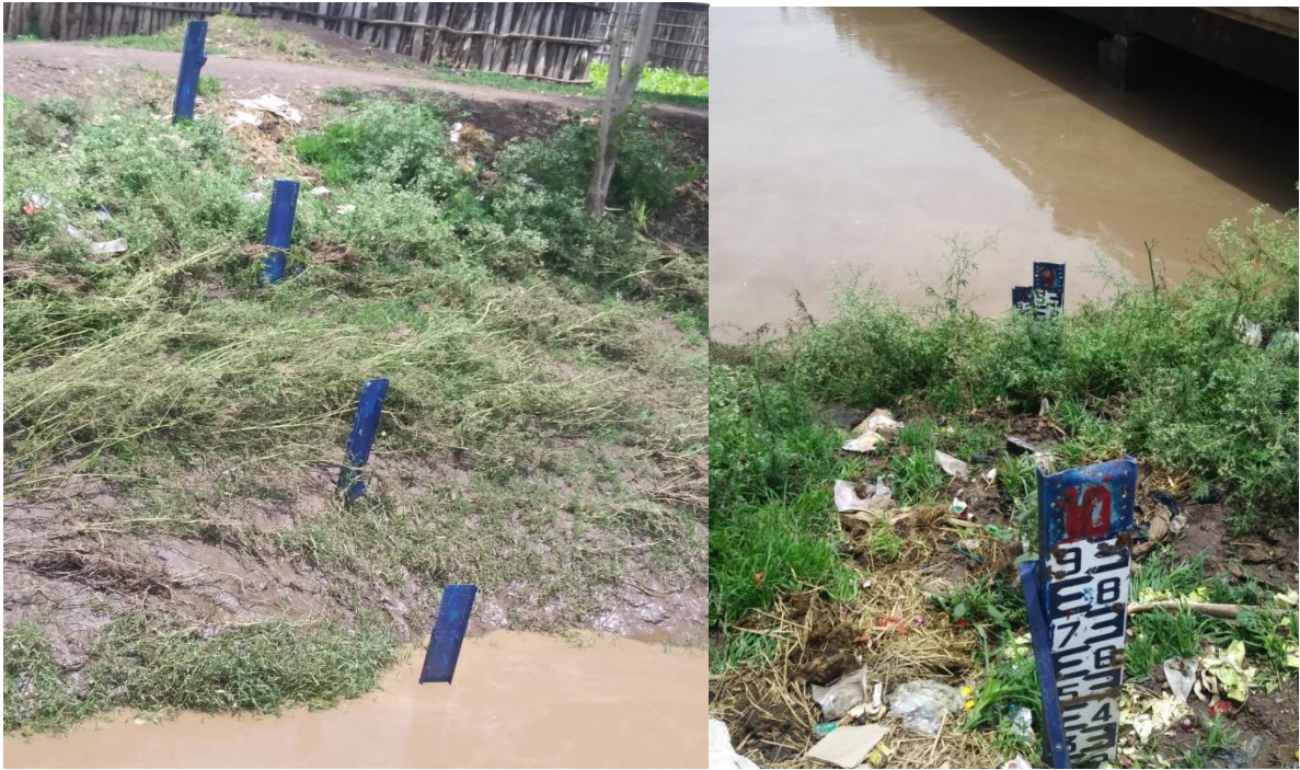
the traditional stream flow measuring instruments used at Ribb River until 4 years ago
