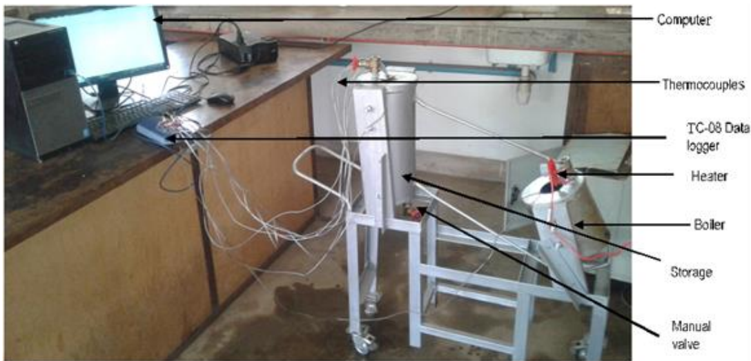
Fig.2: The experimental setup showing charging of the storage tank by thermosiphon principle in which eight thermocouples were connected to a TC-08 data logger to monitor the tanks' temperatures
