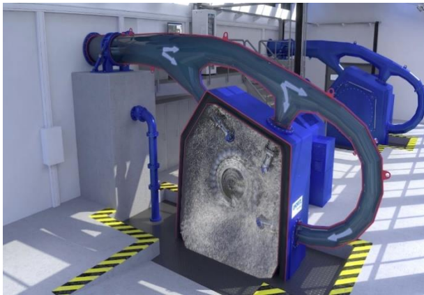
Figure II.10.a: shape of Pelton turbine.
