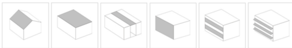
Figure 13: Integration typologies into the building envelope used in IEA Task 41 – Subtask A . From left to right: Tilted roof; Flat roof; Skylight; Facade cladding; Facade glazing; External device.
