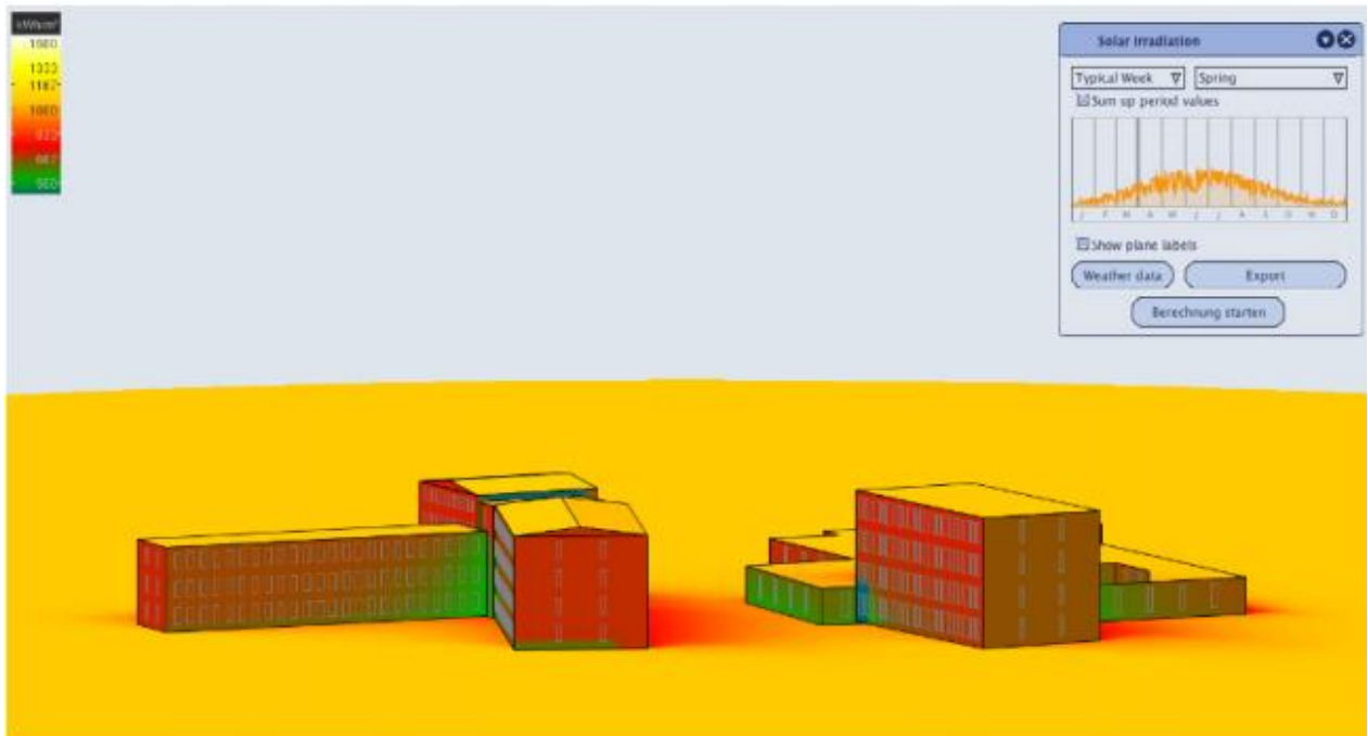
Figure 51: Simulation result for the solar irradiation depicted as a false colour image for a one-year calculation period (Hendel S, Voss K, 2017)
