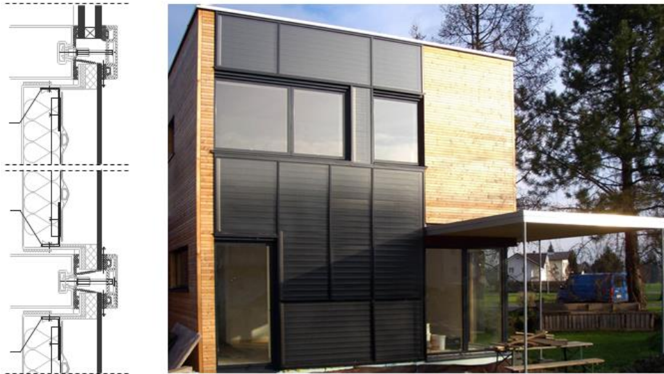
Figure 35: Façade integration of glazed flat plate collectors as façade cladding, detail and picture. (AKS Doma, s.d.)
