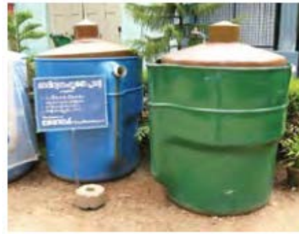
c- Above ground floating drum made of fiberglass reinforced plastic in India
