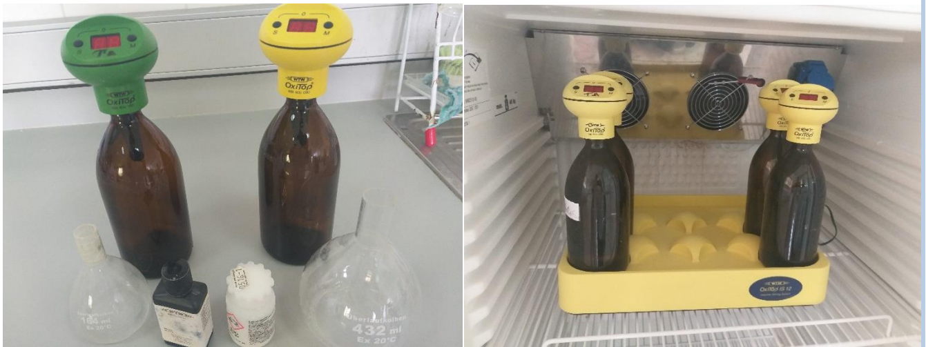
Figure III.5: Biological oxygen demand measurement
