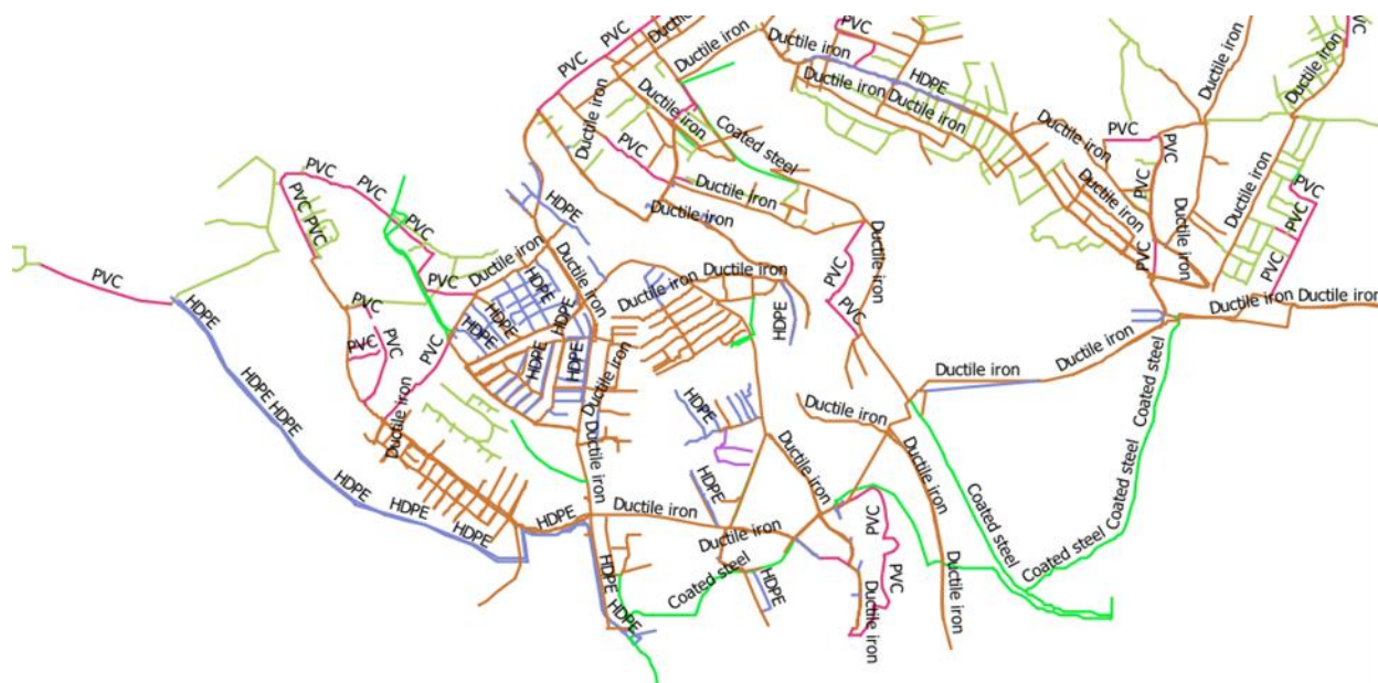
Figure 4.1: Color Coded and Symbology According to Pipe Material of the Ghazaouet Network
