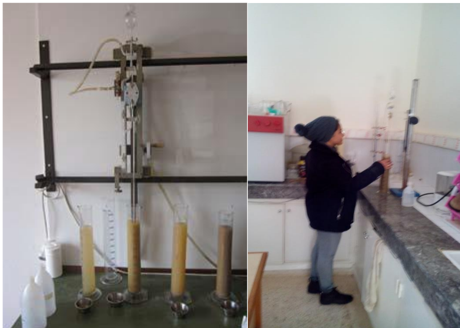
Figure 4-5: Method to separate clay and silt particles (Lab. work).
