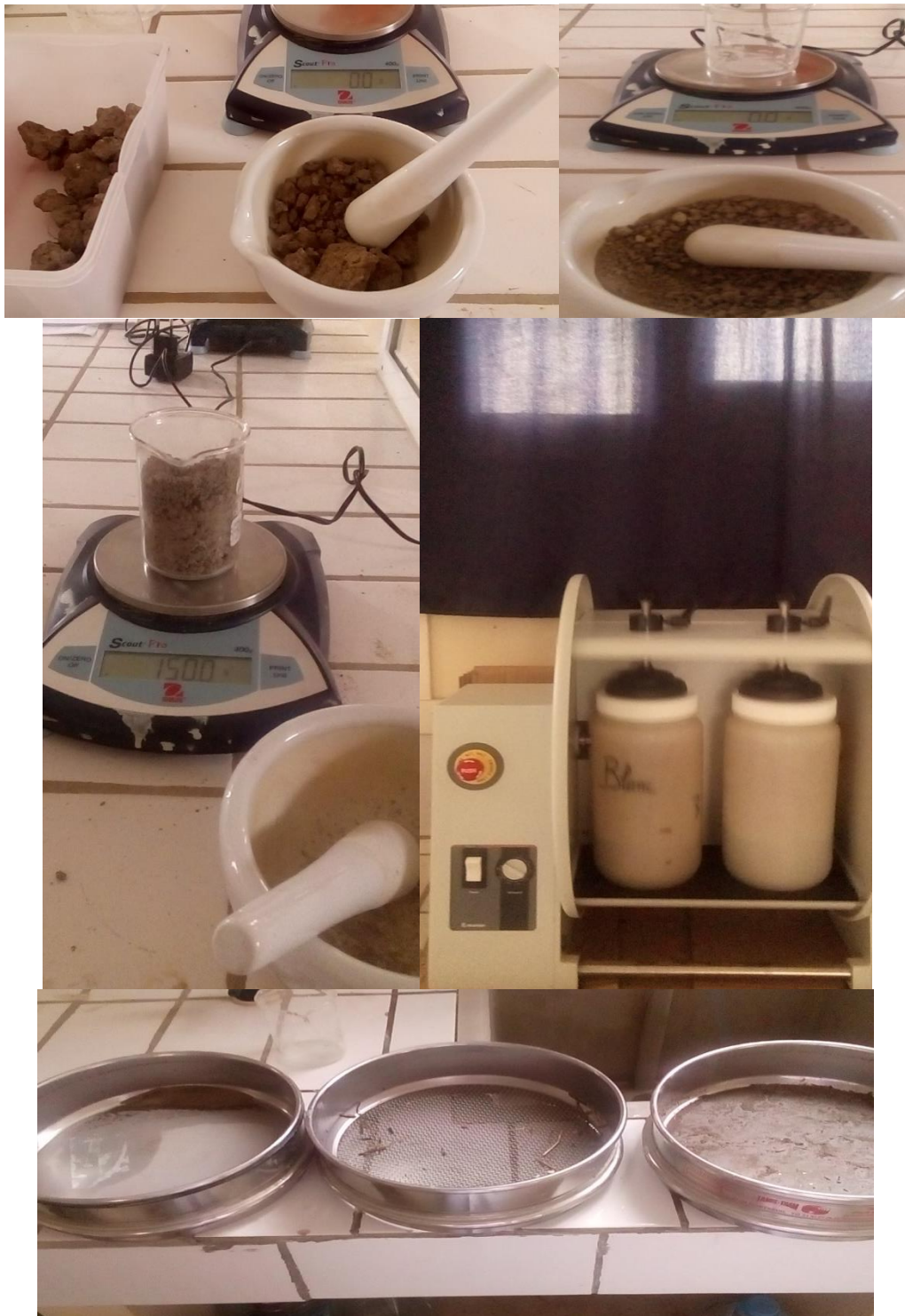
Figure 4-3: wet sieve method analysis.
