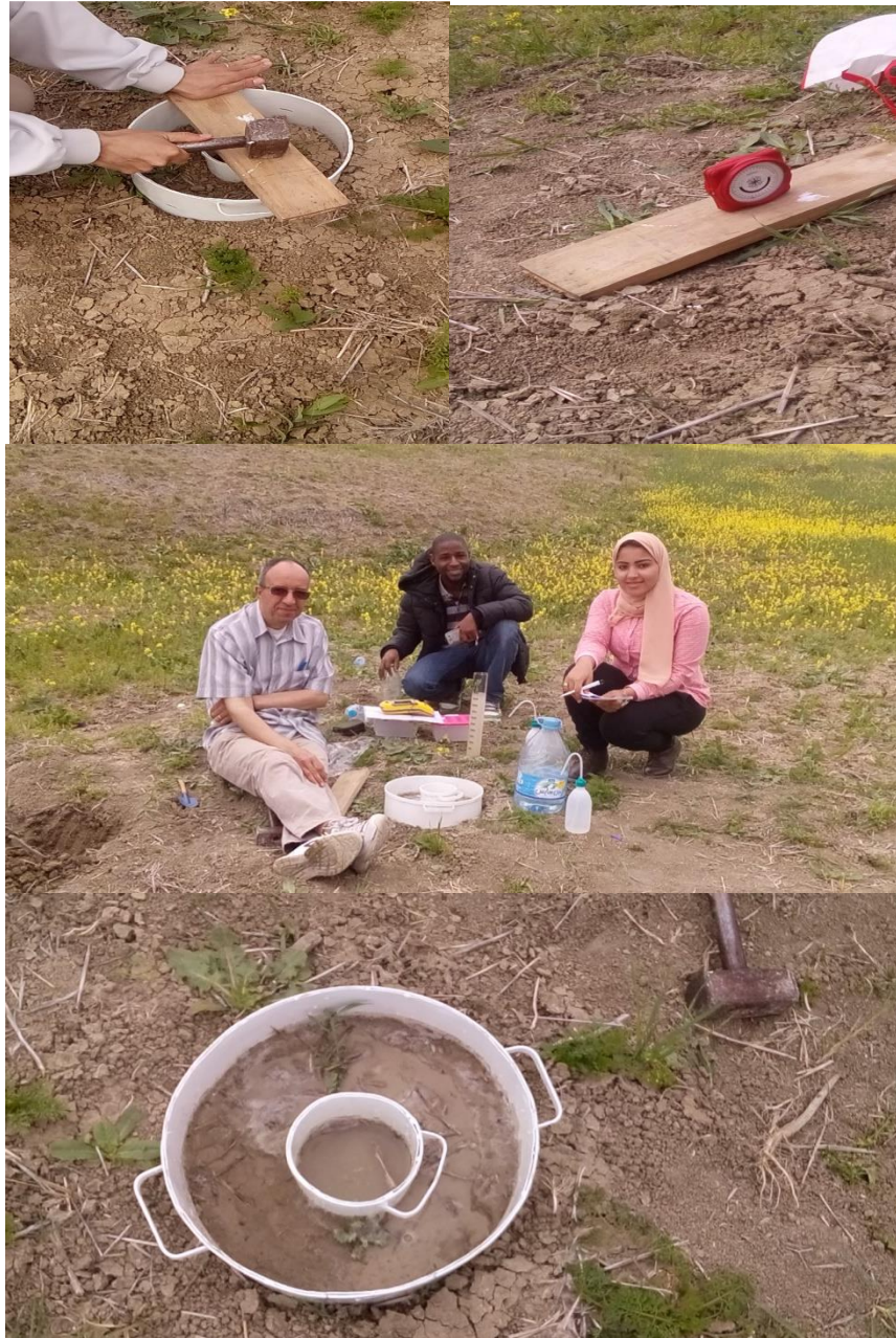
Figure 4-2: Double ring infiltration test (photos from the field).
