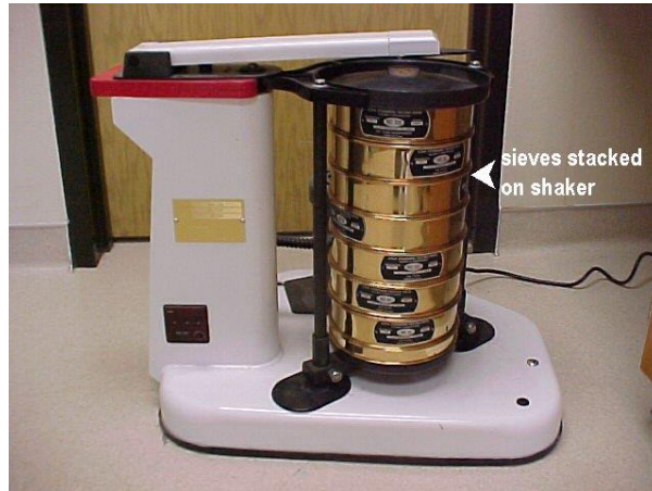
Figure 4-4: Dry Sieve method analysis ( Brittain, 2002 ).
