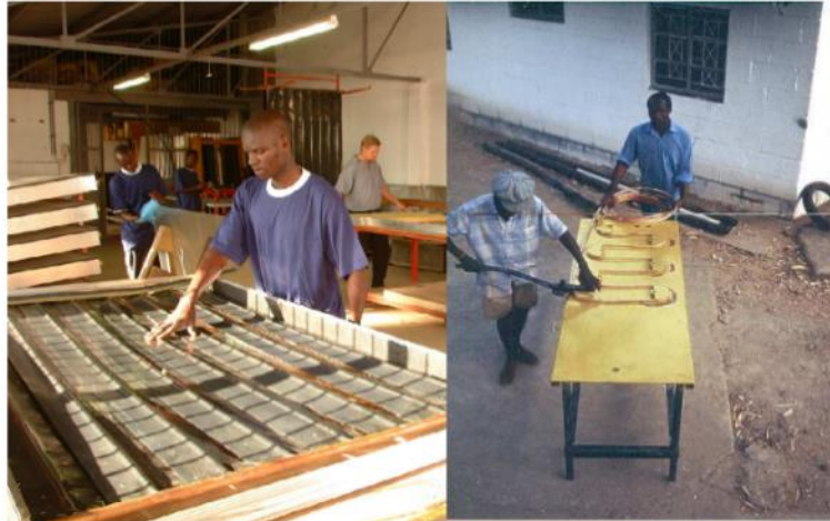
Figure 2. 14: Local production of flat plate solar collectors in Uganda
