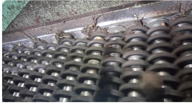
Figure 3. 3: Waste chopping machine
