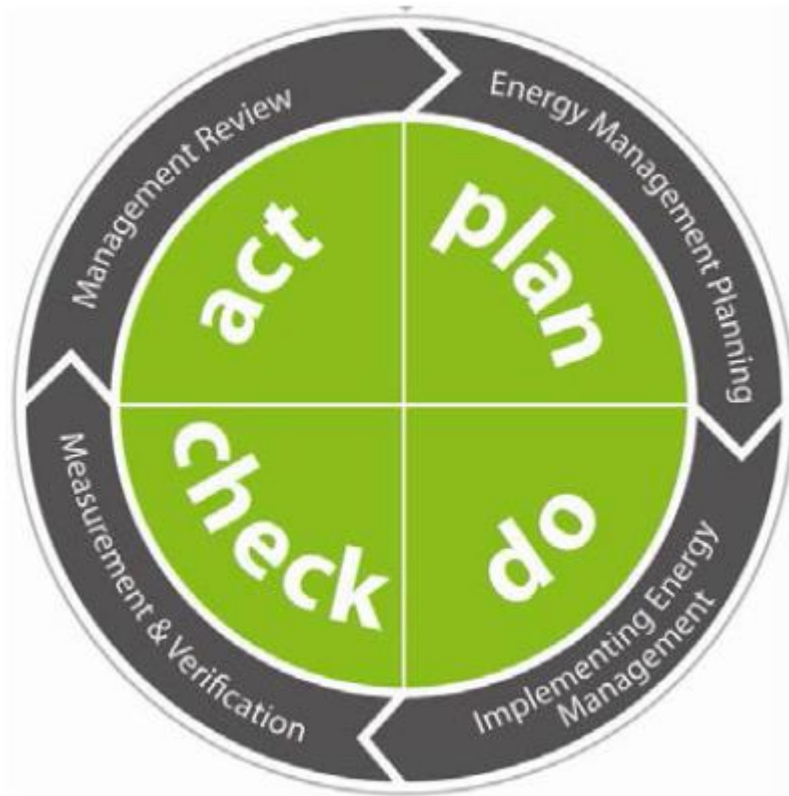
Figure 2.3: Cyclic approach of an energy management system aiming at continued improvements.
