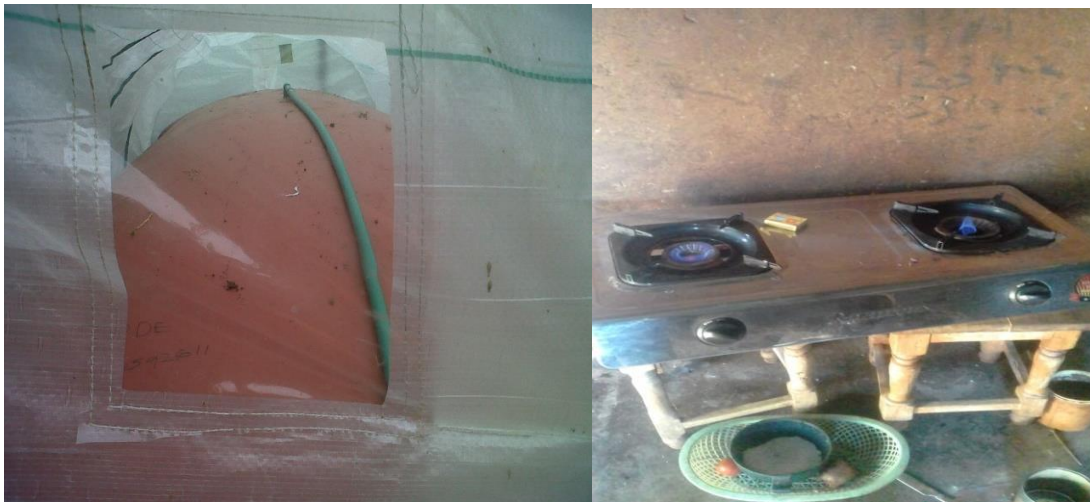
Picture c and d showing components of a small-scale biogas system and burner
