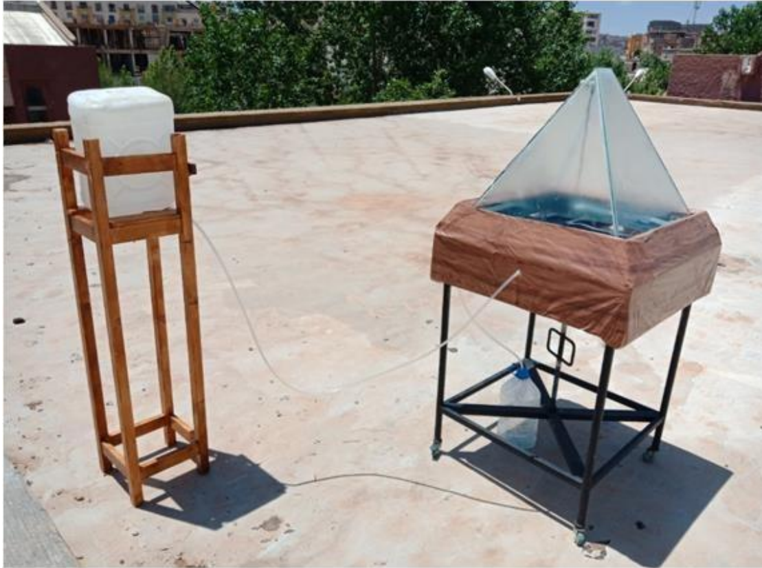
Figure 5-7: Prototype and feeder system of the tank
