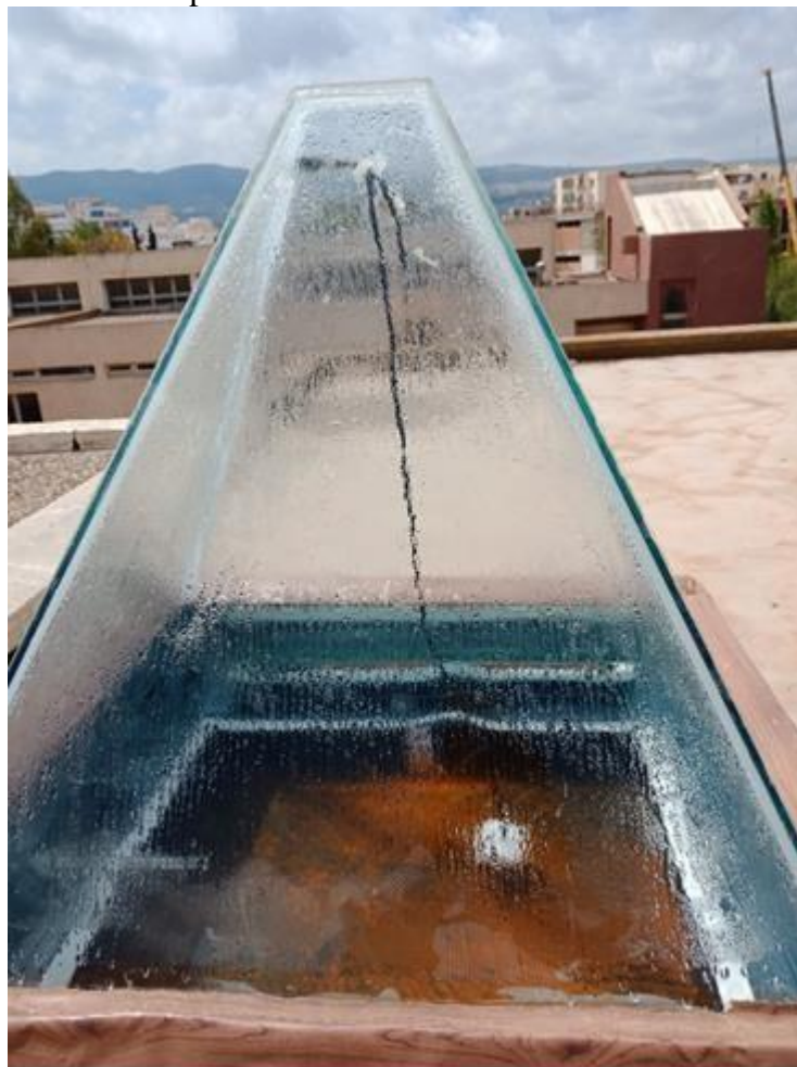
Figure 5-5: Condensation of steam at the top of the prism and on the walls
