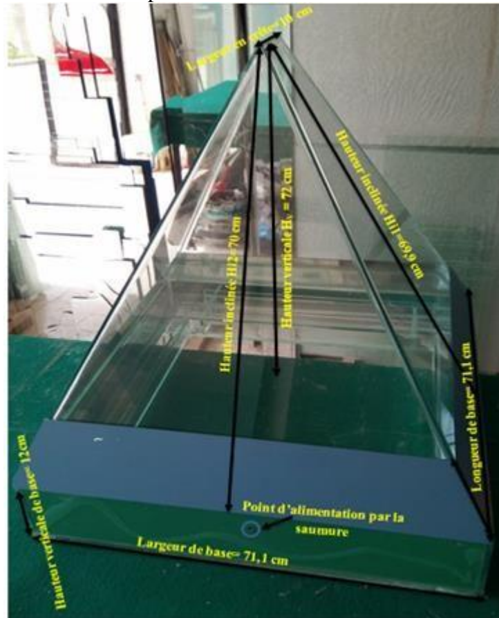
Figure 5-1: Sizing of the glass prism
