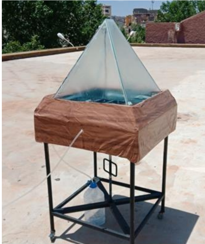
Figure 5-6: Prototype and permeate evacuation system
