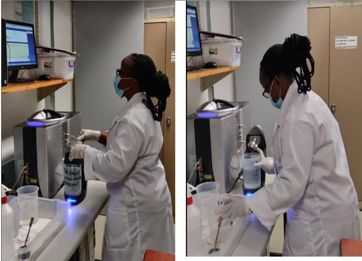
Figure 9: PSD analysis set up using Malvern Mastersizer 3000
