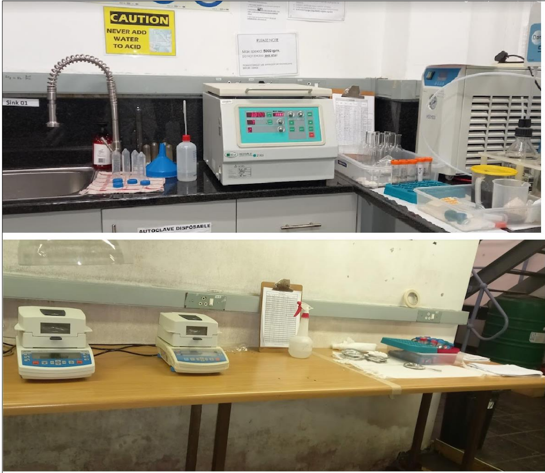
Figure 12: Centrifugation and moisture content analysis set up
