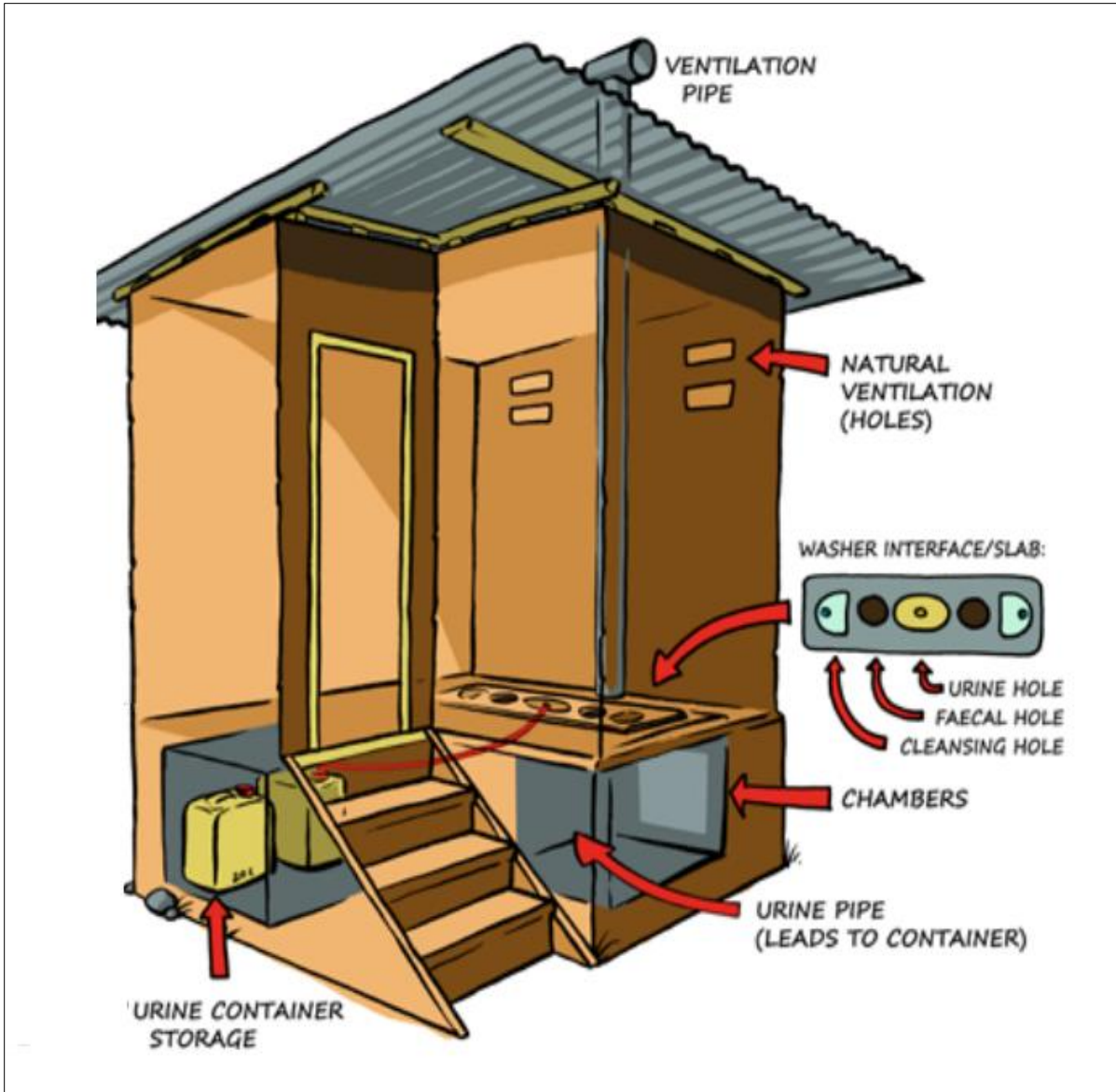
Figure 2: The principle of urine diversion dry toilet (UDDT)
