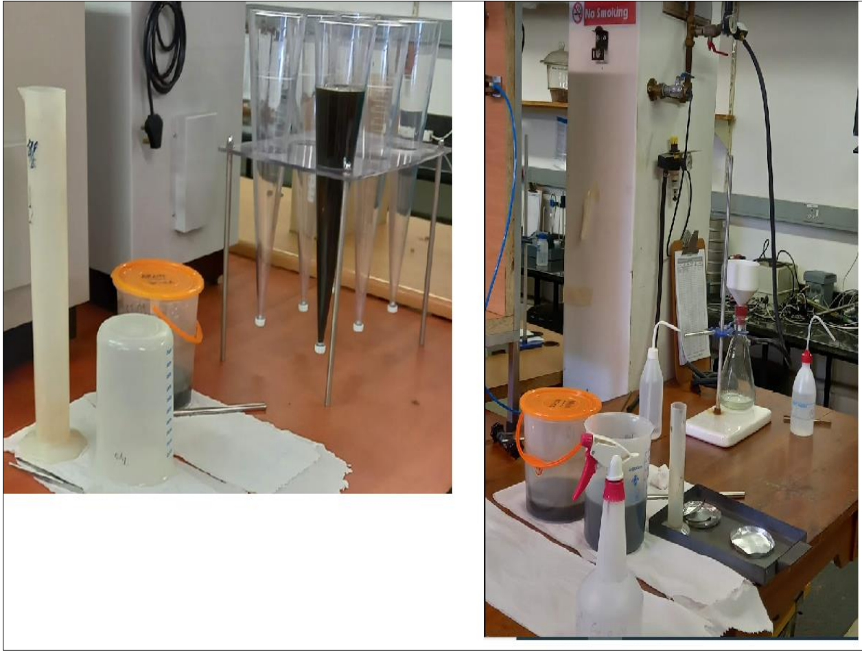
Figure 10: SVI and DSVI laboratory set up
