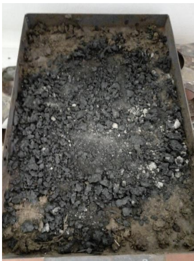
Figure 9 an image of FS after 90 minutes of oven drying at a temperature of 200°C
