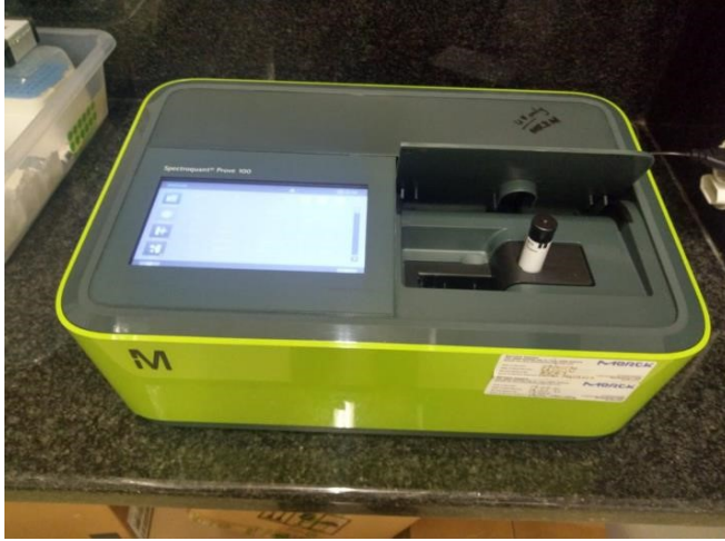
Figure 5: spectroquant machine used to measure nutrient concentration in prepared solutions.
