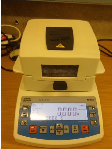
Figure 4: thermal balance machine used for measuring moisture content
