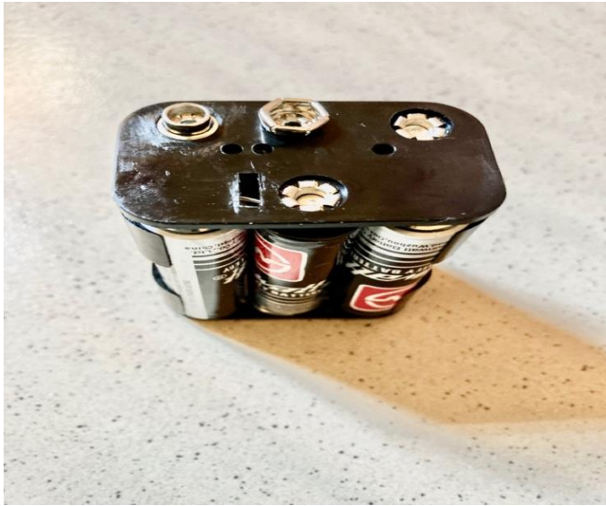
Figure 20. Power supplying batteries: 6 x 1.5 V AA
