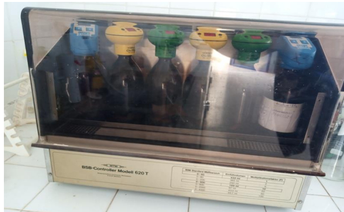
Photo C.5: Biological Oxygen Demand Measurement
