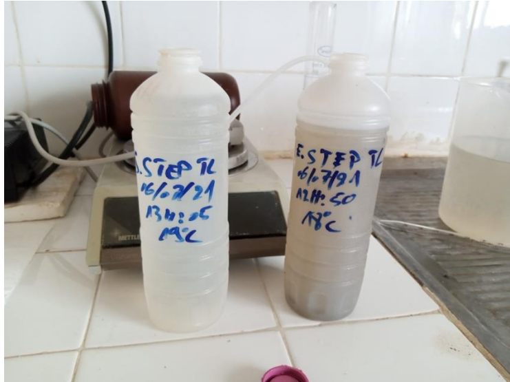
Photo C.8: Samples from the Inlet (left) and Outlet (right) of the WWTP to be Analyzed
