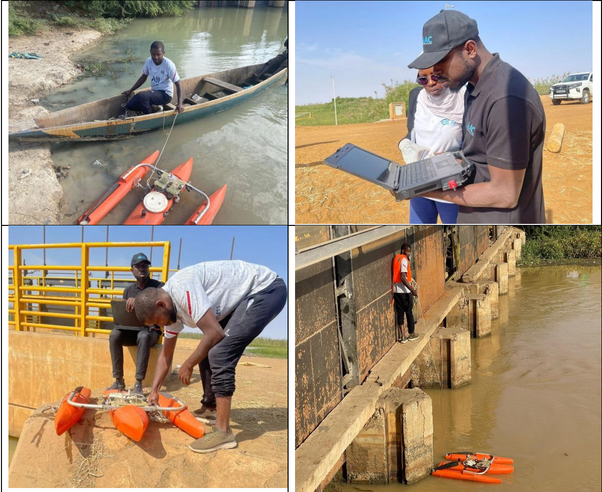
Figure 15: Flow measurement with ADCP
