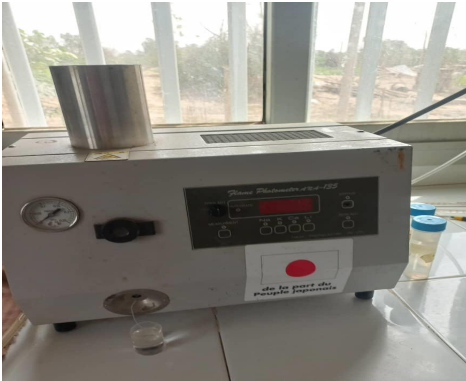
Figure 6: flame photometer for determination Na and K
